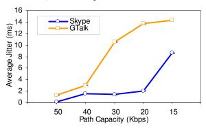
Figure 4 – Average jitter for capacity variation
