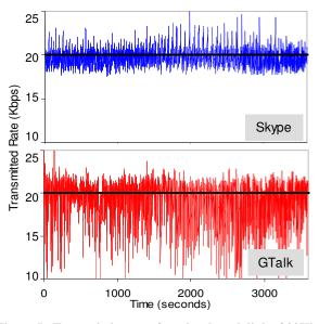
Figure 5 – Transmission rate for a bottleneck link of 20Kbps
