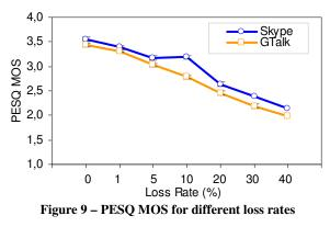
However, these adaptations were not enough to keep the MOS value high (Figure 9). Notably, with the loss rate at 5%, Skype used more redundancy than was necessary, consuming network resources in excess without benefiting significantly its MOS score. We concluded it by observing that with the loss rate at 10%, the MOS value didn't change.
