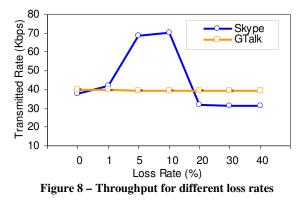
Figure 8 shows that Skype adapted at various levels of loss, while GTalk behavior indicates it has no mechanism of adaptation to packet
