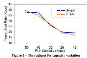
Observing the transmitted rate (Figure 2) and PESQ MOS results (Figure 3), it is possible to observe that when the capacity of the network path is 50Kbps GTalk utilizes more bandwidth, transmitting at a rate higher than Skype, but obtains the same audio quality (the
