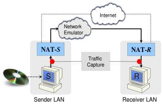
Figure 1 – The testbed for the experiments
