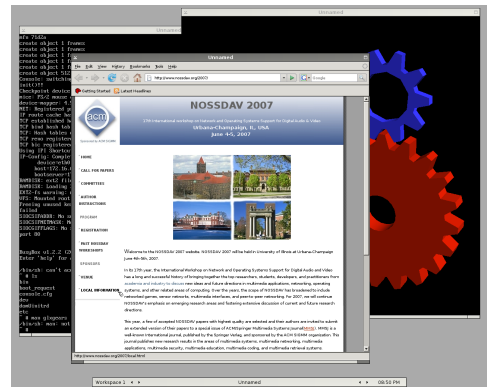
Figure 4: Blink running in root-less mode on top of X11. Here, the kernel framebuffer is shown, both running a text mode console and with X11 in a VM, running a web browser.
